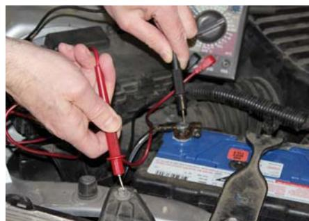
You also need to check the voltage between the negative battery post and the chassis.
