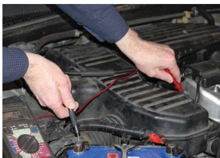
The most basic voltage drop check is between the negative battery post and the engine.
