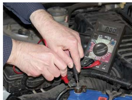
If there is a voltage drop, then you can determine where the fault lies by checking the under-load voltage at various points of the cable. Here we are checking the voltage between the negative battery post and the negative terminal.
