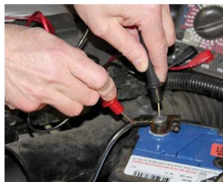
If you are still chasing the source of the voltage drop between the battery and the engine or chassis, then check the drop between the conductor and the battery post.
