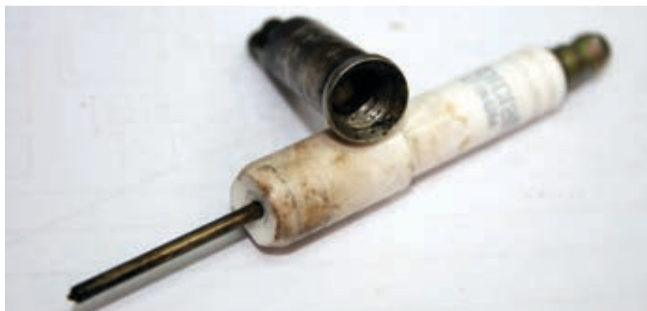
Diagram #2 Spark Plug after removal using Special Tools
